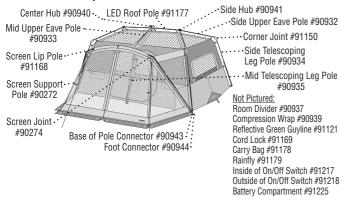
Empty contents of bag and confirm all parts are included and undamaged.
